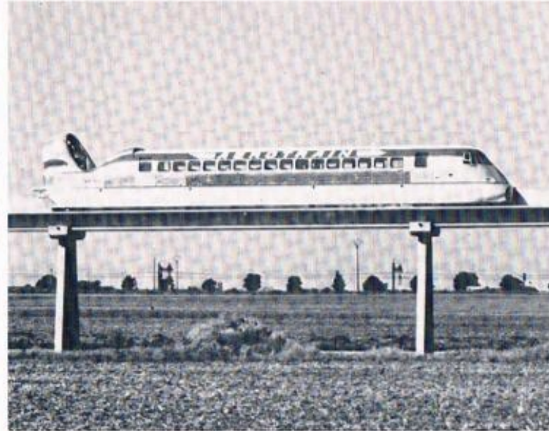
Eighty-passenger air-cushion vehicle in operation near Orleans, France. Speeds up to 265 miles per hour have been reached by Aerotrain test vehicles.
