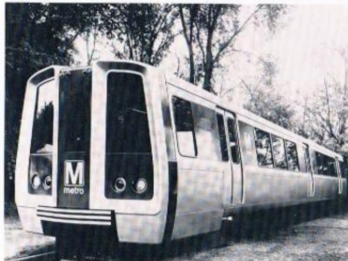
Aluminum rapid transit car for new Washington, D.C. Metro System. Rohr has a contract to build 300 cars at its Winder, Georgia assembly plant.
