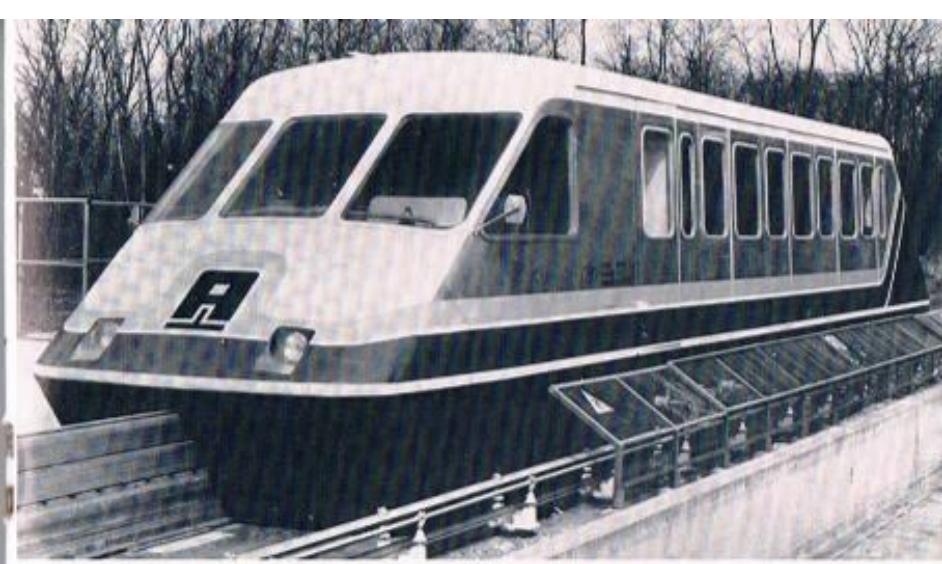
A 44-passenger TACV being demonstrated near Paris with a linear-induction motor. Rohr's Aerotrain Systems subsidiary has drawn upon the French technology.
